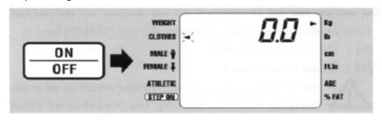
Press ON/OFF key to turn the machine on. Wait until 0.0 and an arrow appear on the screen. Check that the arrow points to "Kg". If arrow point to "lb", press the Kg/Lb key on the control panel and the arrow will shift to "Kg"
