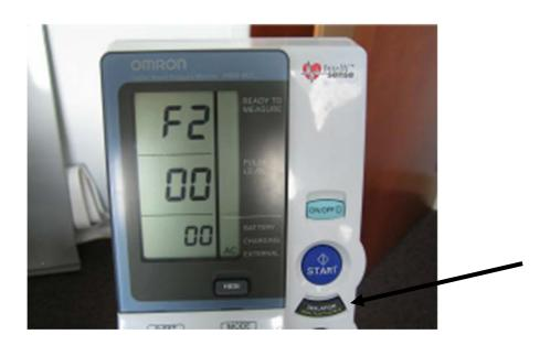
If needed push the DEFLATION (deflation control)/Measurement Result Display Switch Button and change the set value to 0 sec waiting time. Push the START button and F3 function is displayed in the first window and inflation interval 30 second time is displayed in the bottom window (Figure 13.8).
