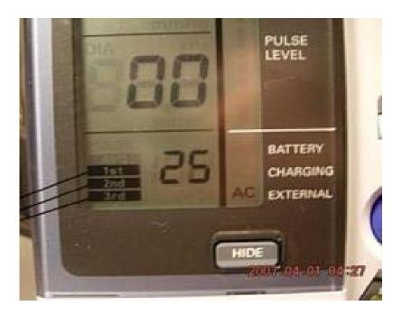
After each inflation and deflation, the systolic blood pressure, diastolic blood pressure and pulse rate will be displayed in the top, middle and bottom sections of the LCD screen.
