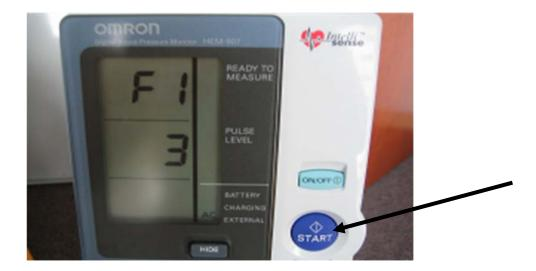
Push the START button and F2 function is displayed in the first window and 0 waiting time is displayed in the middle window (Figure 10.7)
