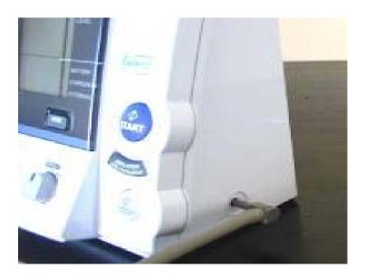
For all cuff sizes small, medium, large, and X-Large connect the air tube to the main unit by attaching the air plug to the base of the air connector. Connect the cuff to the air tube attached to OMRON unit Wrap and secure the appropriate cuff to the participant's upper right arm as set out in section 10.2.7, above.
