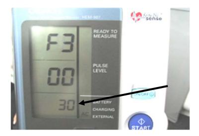
If needed push the DEFLATION (deflation control)/Measurement Result Display Switch Button and change the set value to 30 sec measurement interval.
