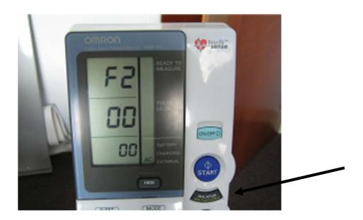
If needed push the DEFLATION (deflation control)/Measurement Result Display Switch Button and change the set value to 0 sec waiting time. Push the START button and F3 function is displayed in the first window and inflation interval 30 second time is displayed in the bottom window (Figure 10.8).
